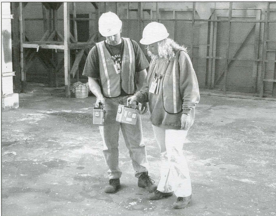
Environmental scientists compare Geiger counter measurements during radiological investigations at Hunters Point Shipyard.
