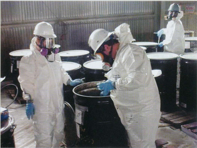
Above: Environmental technicians collect samples from waste materials remaining in Building 369 for analysis.
